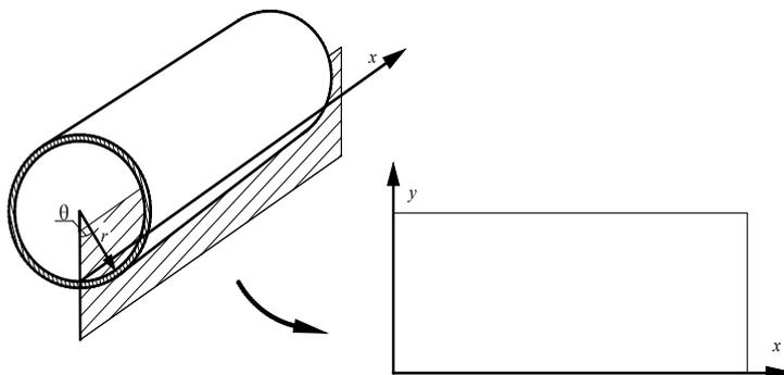
Figure 2. Using cutting and unrolling to turn the tunnel to 2-D
