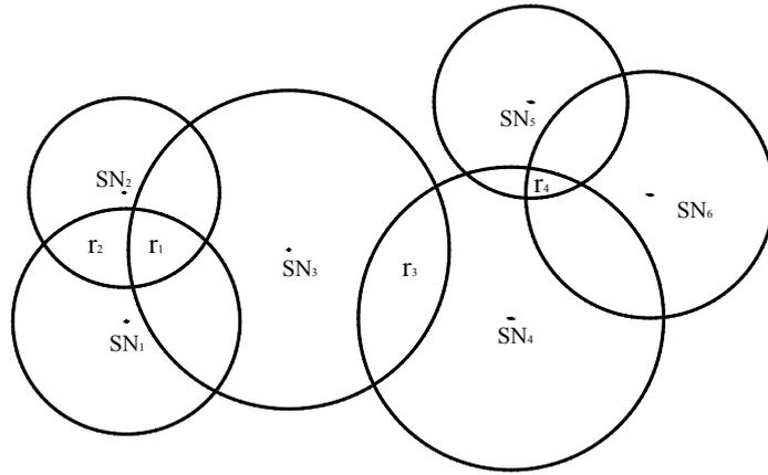
Figure 3. A set of SNs and their transmission radius,  $r_i$  denotes the overlapping regions
