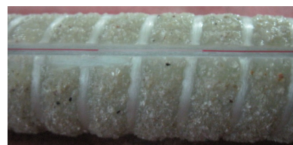
Figure 6. GFRP bar Built-in FBG
