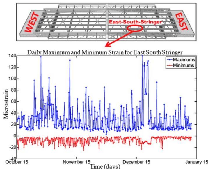
Figure 3. Daily maxima and minima strain for each day from East South stringer
