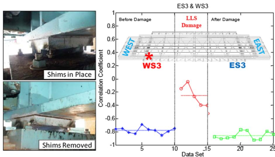
Figure 5. LLS shims and correlation coefficient change before, during, after damage
