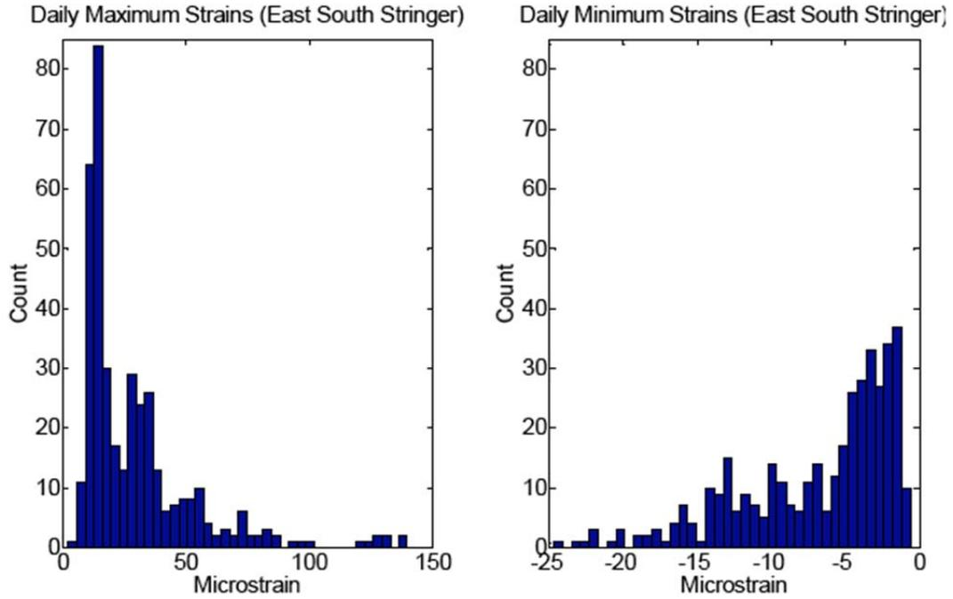
Figure 4. Three months strain data histogram from East South stringer
