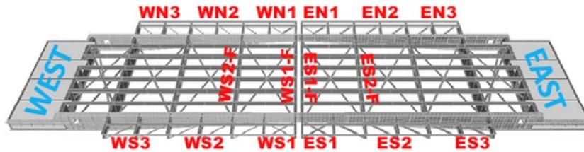
Figure 2. Instrumentation plan for the high-speed strain measurements on structural components
