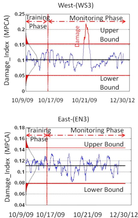
Figure 6. Moving Principle Component Analysis (MPCA) results related to a sensor close to damage location (WS3) and a sensor far from damage location (EN3)
