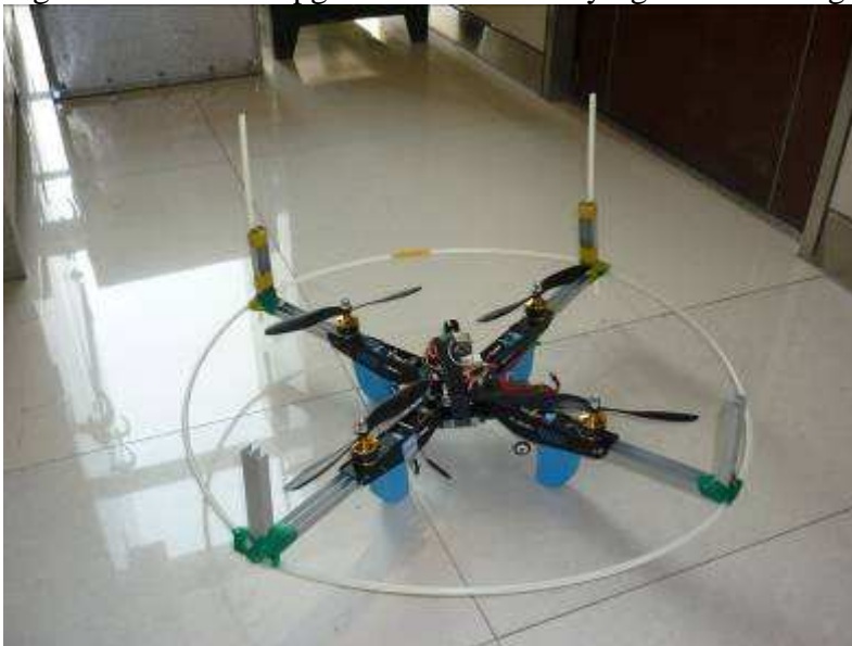
Figure 7 The structure of the upgraded UAV for staying on the side.
