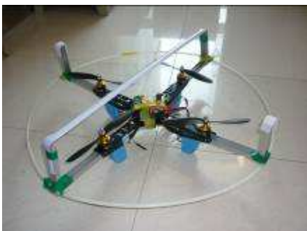
Figure 4 The structure of the upgraded UAV for staying on the ceiling.
