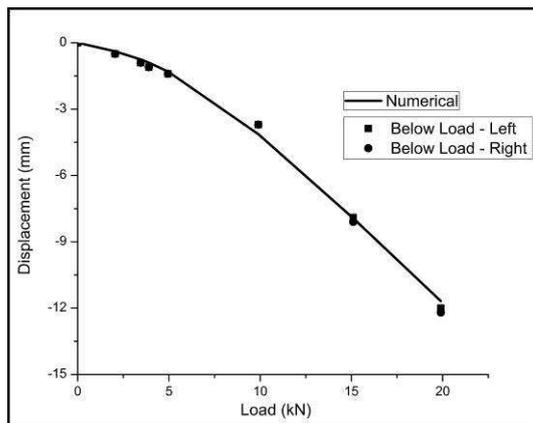
Figure 10. Results for displacement measurements below load application point
