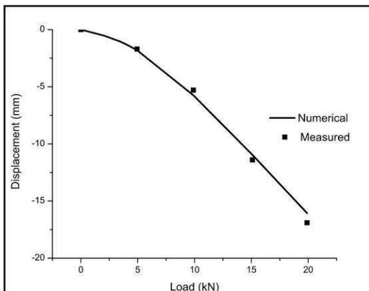
Figure 9. Results for displacement measurements at centre of span
