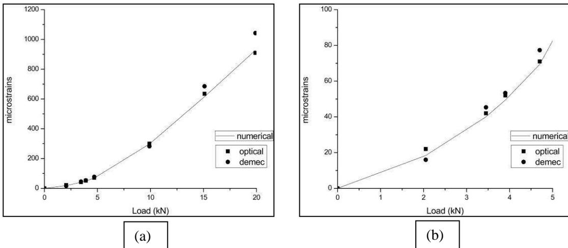
Figure 8. Results for Concrete Strain Measurements – a) Full Range and b) For 5 kN
