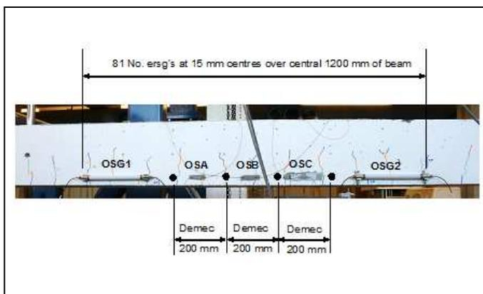
Figure 2. Sensor placements on the test beam
