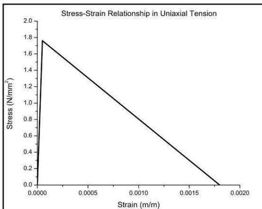
Figure 6. Concrete Tensile behaviour as determined by best fit of results to experiments
