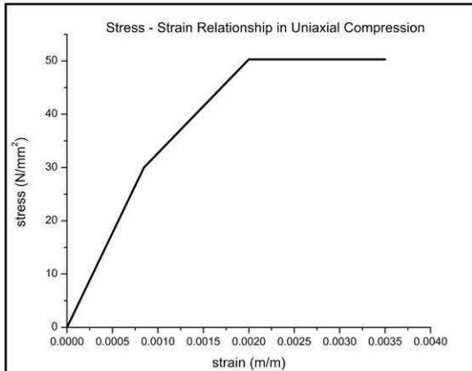
Figure 3. Compressive stress-strain relation in concrete
