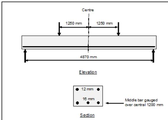
Figure 1. Description and Layout of the test beam
