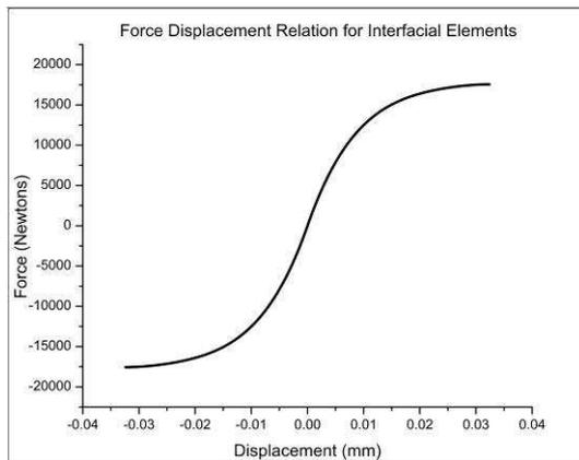
Figure 5. Bond behaviour between concrete and reinforcement
