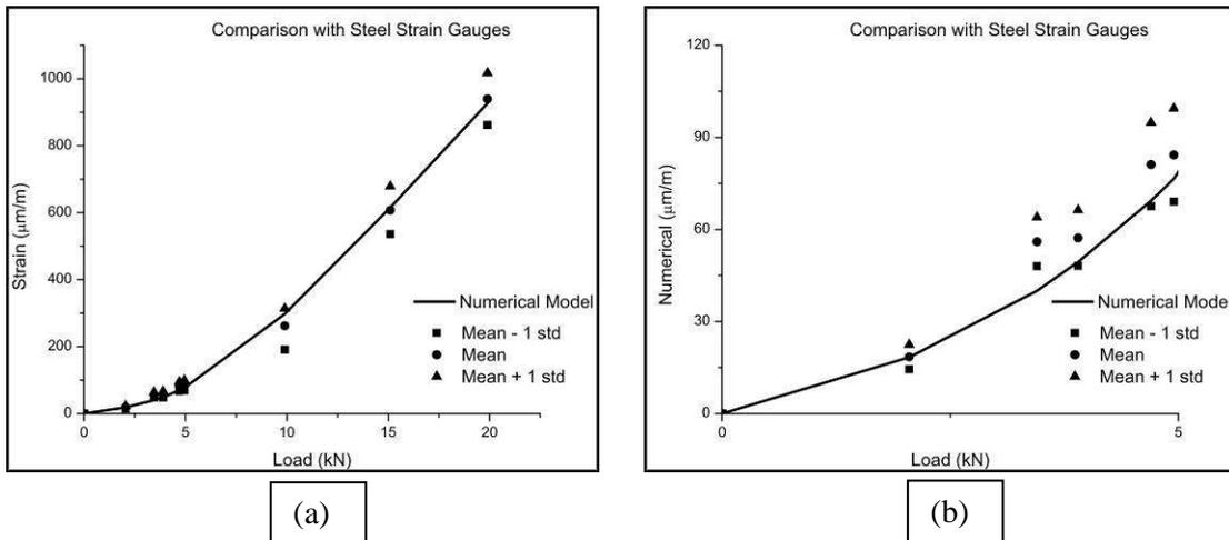
Figure 7. Results for Steel Strain Measurements – a) Full Range and b) For 5 kN
