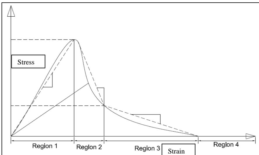
Figure 4. Tensile stress-strain relation in concrete
