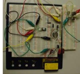
(b) Energy harvesting circuit on a breadboard
