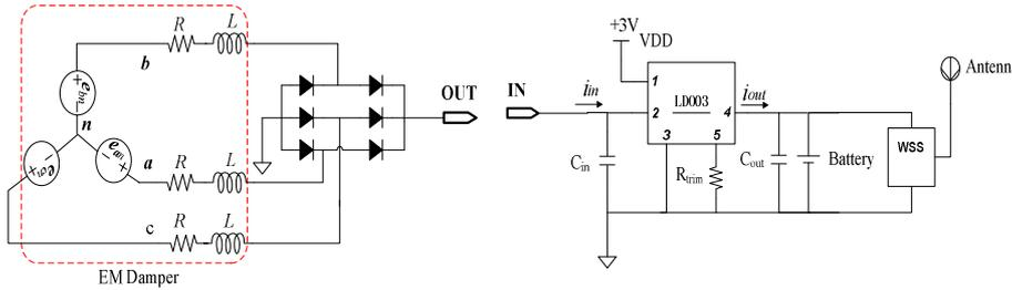
Figure 3 Energy harvesting circuit with a DC-DC converter
