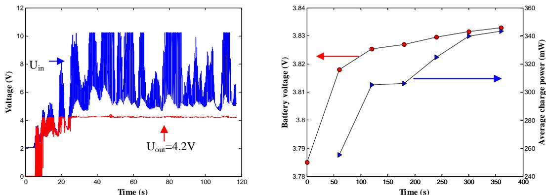
(a) Input and output of Buck-boost converter without load (b) Battery voltage and average charge power
