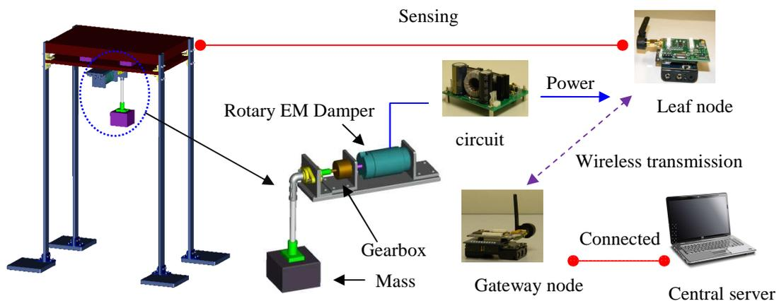
Figure 1. Regenerative EM-TMD system with wireless sensor
