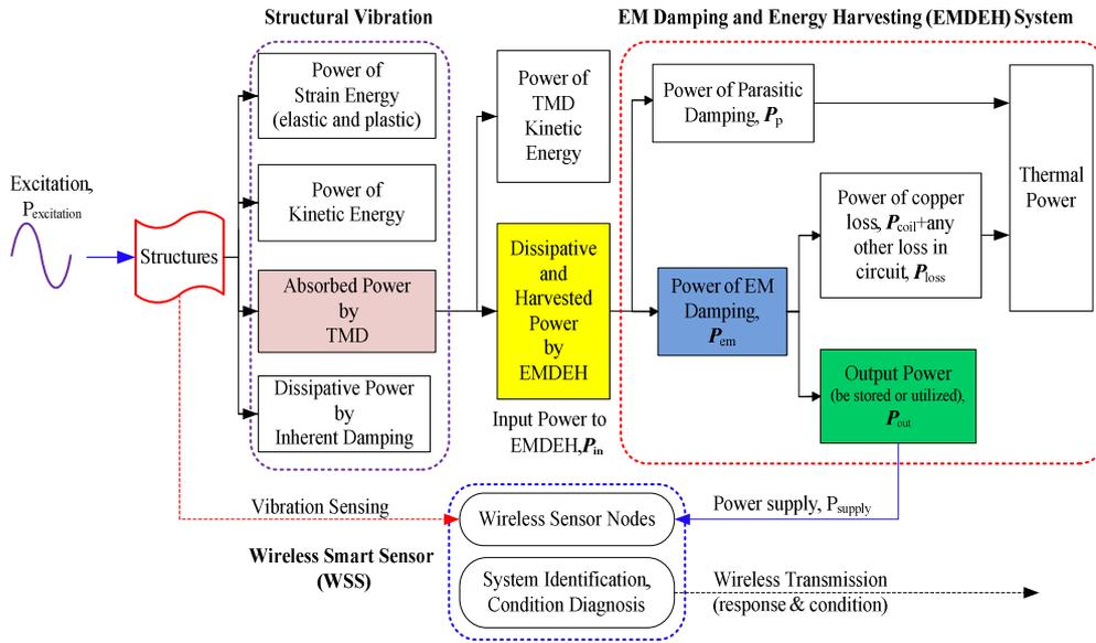
Figure 2. The power flow in a structure equipped with the EMTMD-EHC-WSS system
