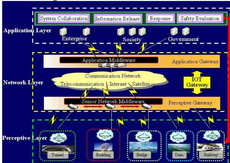
Fig 1. The behavior monitoring IOT system based on smart tags
