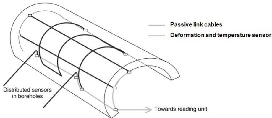
Figure 7. Schematic example of tunnel integrity monitoring
