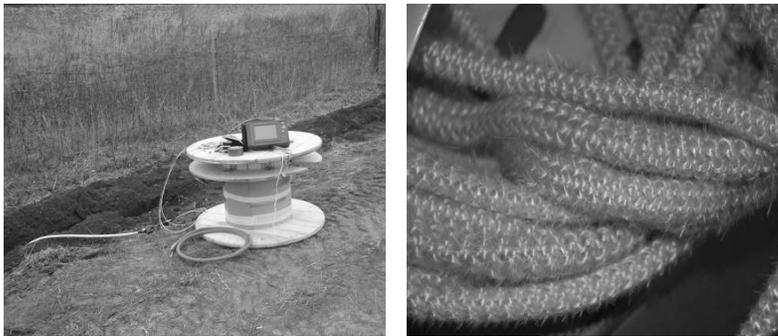
Figure 6. SMARTGeoTex Rope, left, site-installation, right
