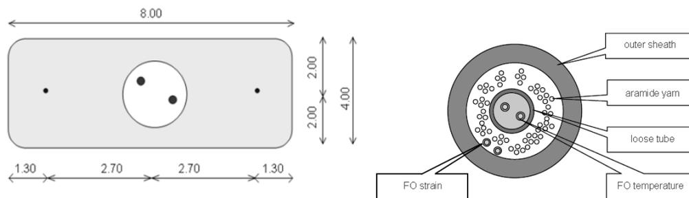
Figure 3. SMARTprofile FOS, right, and SMARTTube FOS, left
