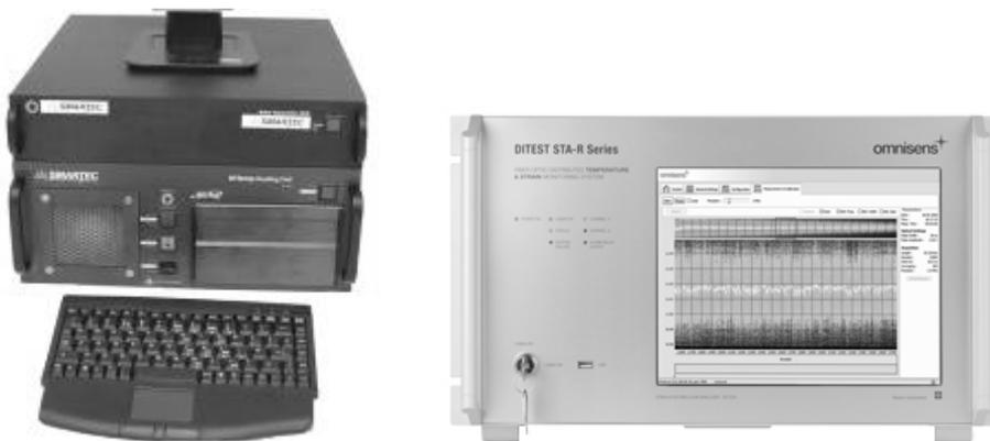
Figure 1. DiTemp (Raman), left, and DiTeSt (Brillouin), right, distributed read-out units
