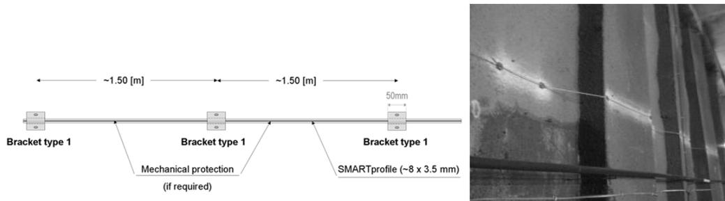
Figure 8. SMARTprofile FOS surface installation
