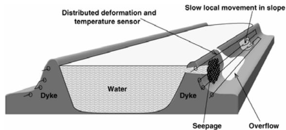
Figure 4. Schematic representation of distributed deformation and temperature FOS locations in a levee for seepage and overflow detection (distributed temperature FOS) and localization of slow slope movements (distributed strain FOS)
