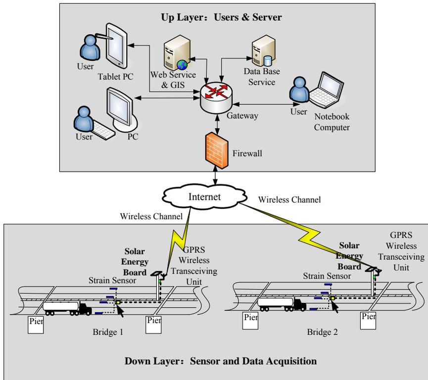
Figure 1 The functional block diagram of the distributed wireless bridge monitoring system in Hangzhou
