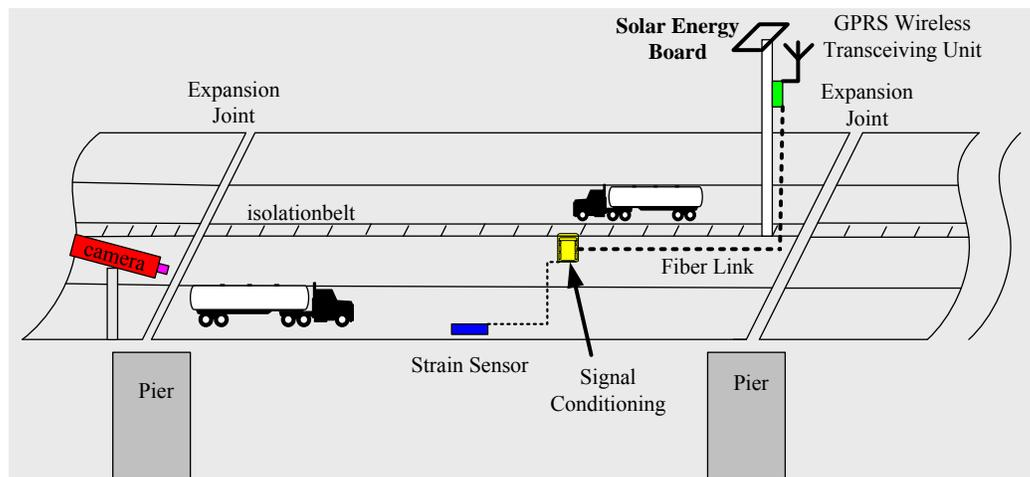
Figure 7 The schematic diagram of the installation of the sensors and cameras at the system testing field.
