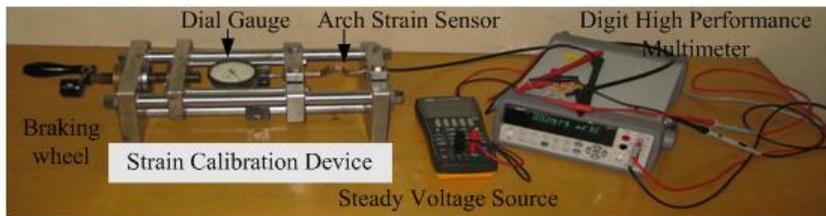
Figure 5 The strain sensor marking system
