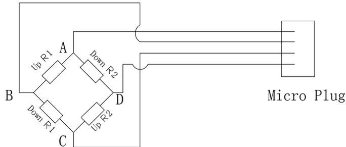
Figure 4 The circuit of the bridge strain sensor
