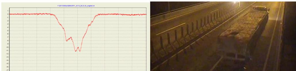
Figure 8 (f) Time: 0:23:56; Maximum variation of stresses: 29; Kind of Vehicle: truck of 6 axles
