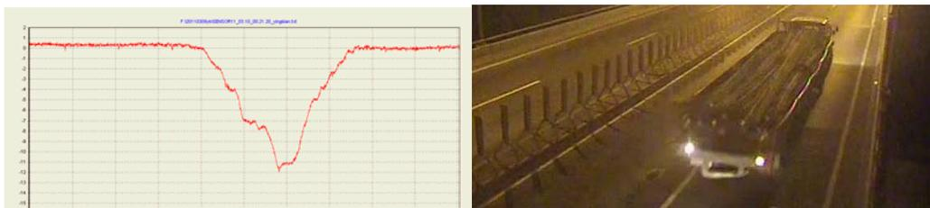
Figure 8 (e) Time: 0:21:45; Maximum variation of stresses: 30.5; Kind of Vehicle: truck of 6 axles
