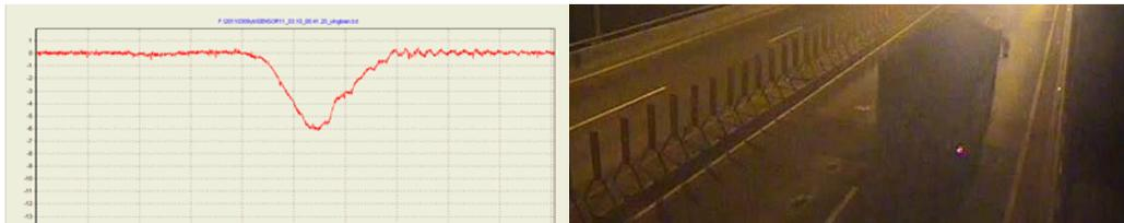
Figure 8 (d) Time: 0:42:01; Maximum variation of stresses: 15.5; Kind of Vehicle: truck
