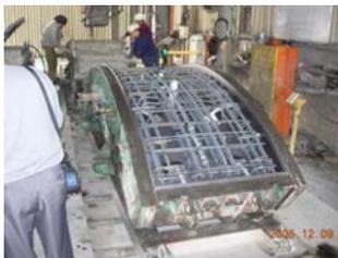
Figure 5. Installing the SOFO sensor system on the cage bar
