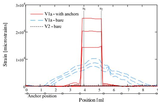
Figure 4. Comparison of V1a / V2 in 0.1m depth
