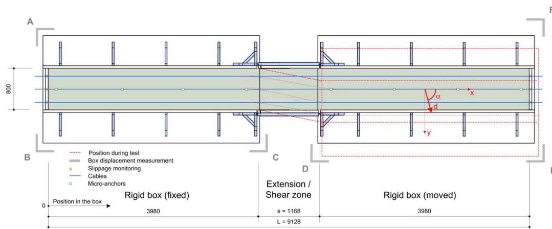
Figure 3. Test setup, dimensions in [mm].
