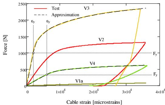
Figure 1. Tension test results,  $\dot{\varepsilon} = 2300 \mu\varepsilon/\text{min}$ .
