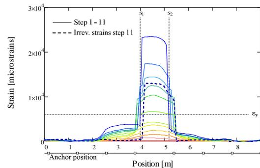
Figure 6. V4 cable with anchors in 0.5m depth.
