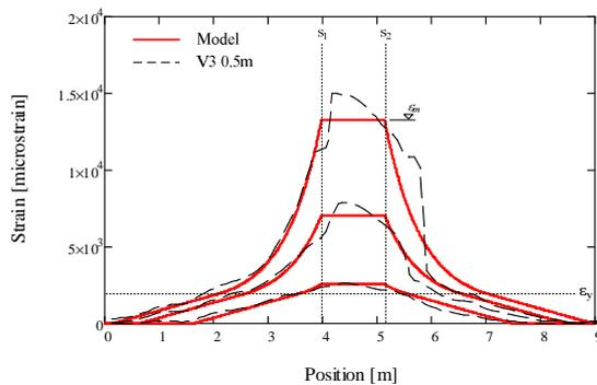
Figure 13. Comparison Model – Test for V3 0.5m.
