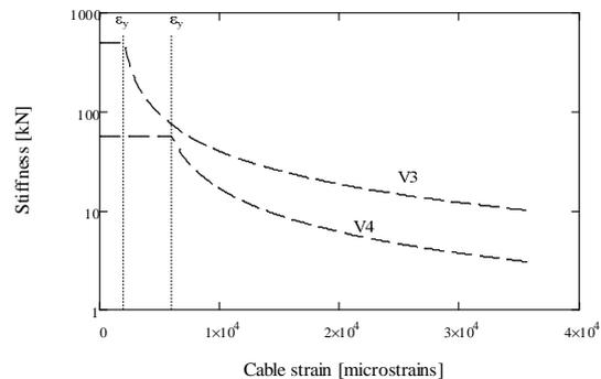
Figure 2. Tangent stiffness for V3 and V4
