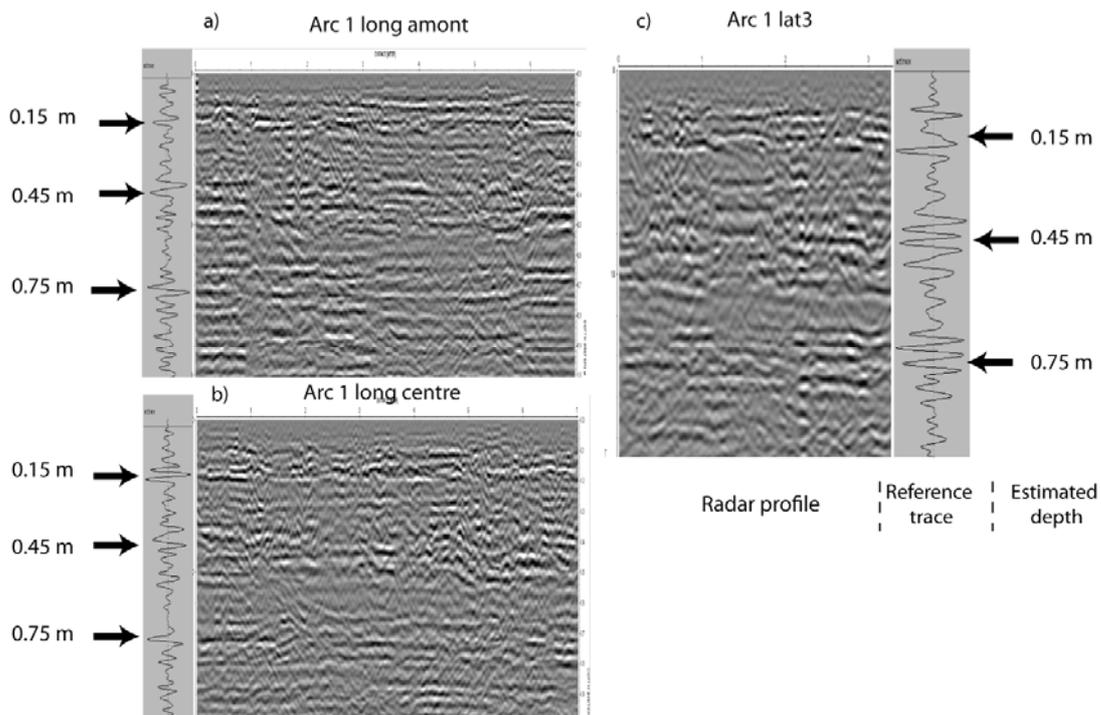
Figure 5. Radargrams of the arch 1: a) and b) longitudinal profiles, c) transversal profile
