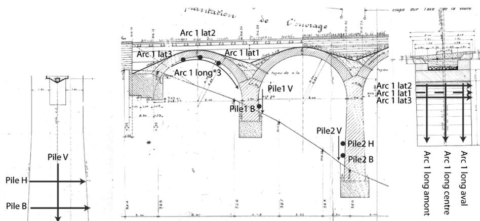
Figure 3. GPR profile measurements
