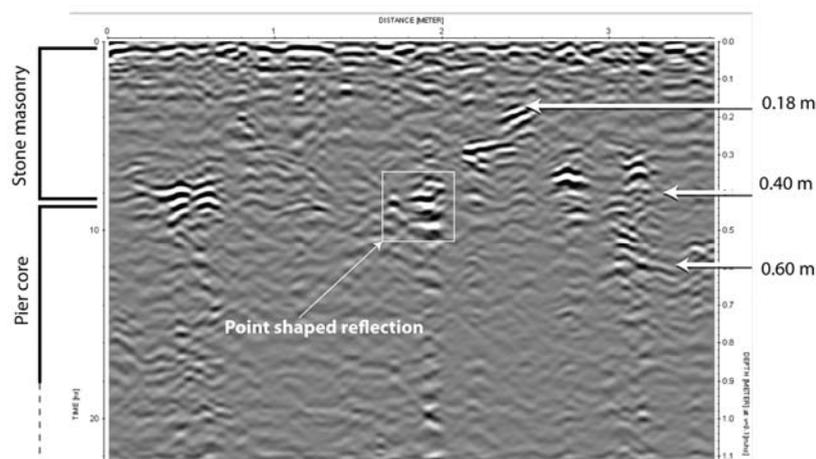
Figure 4. Radargram at the base of the second pier (i.e., Pile2 B)
