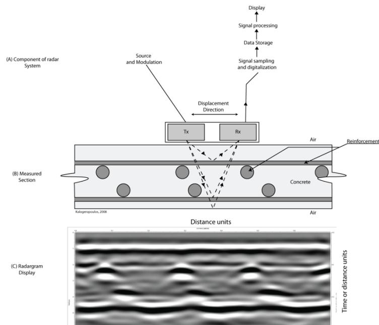
Figure 1. Principle of a GPR measurement.
