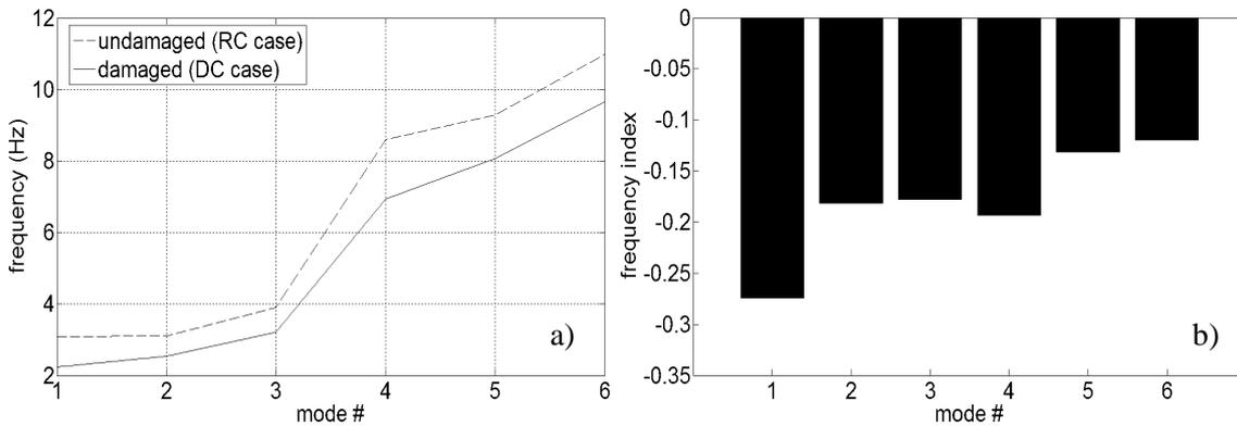
Figure 4: a) – Frequencies for the RC and DC cases; b) – Frequency index for all modes.
