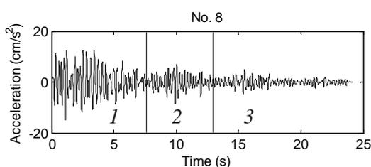
Figure 6. Typical structural responses of floor 6 under each seismic excitation
