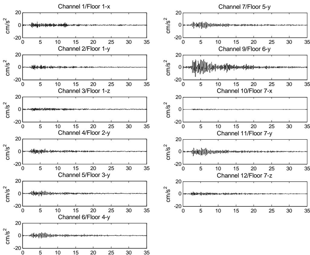
Figure 5. The time history of the No. 8 earthquake and the corresponding structural responses
