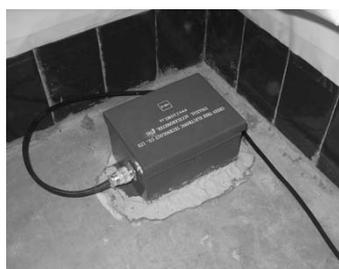
(a) The force-balance accelerometer
