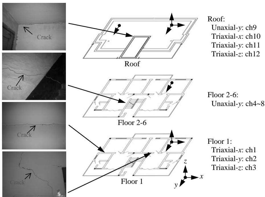
Figure 2. Damage situation of the building and the sensor locations
