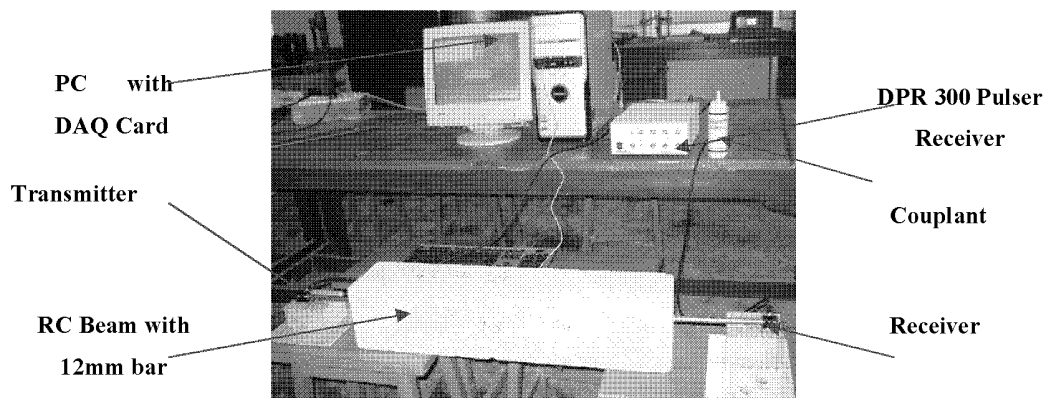
Figure 2. Experimental Set Up for Pulse Transmission monitoring of RC Beams
