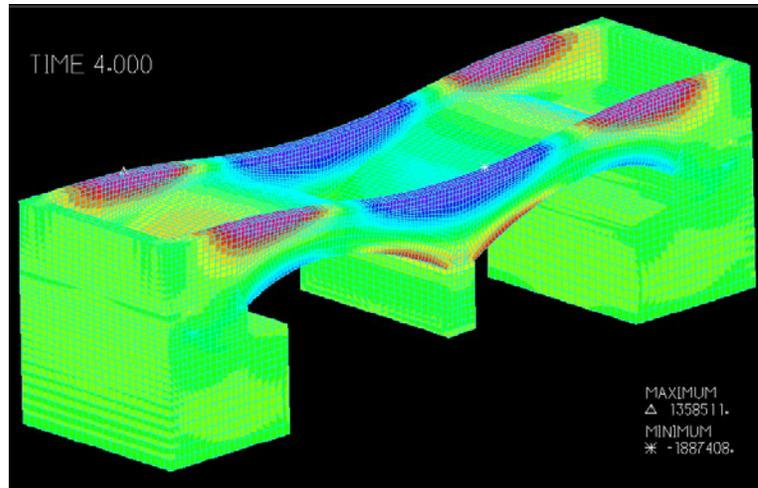
Figure 2 – Preliminary arch bridge FE model
