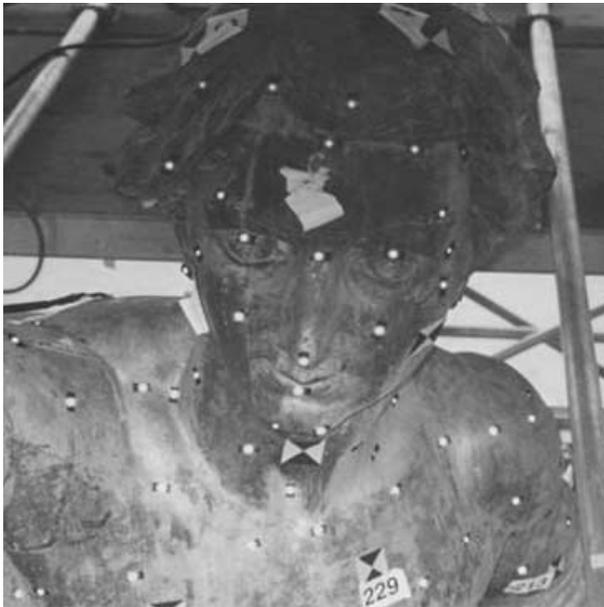
**Fig. 10.** Complex model developed from reflective tape coordinates.
