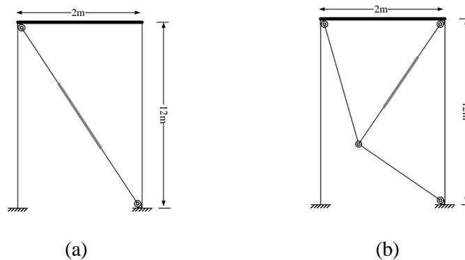
Fig. 6. Frame structure with brace damper subject to earthquake excitation: (a) diagonal brace-damper system; and (b) upper toggle brace damper system.
