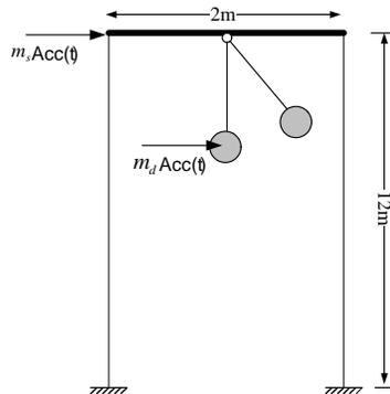
Fig. 3 A frame structure equipped with TMD.
