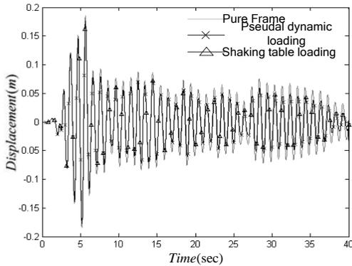
Fig. 7 Comparison of analytical responses of linear diagonal brace damper frame and pure frame subjected to pseudo dynamic and shaking table type loadings.
