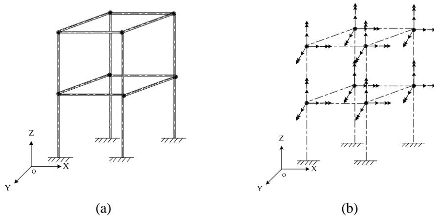
Figure 1 (a) A space frame structure, (b) Discrete particles modeling of a space frame structure system by the VFIFE method.
