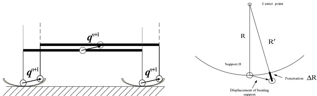
Fig. 5. Modeling of the Friction Pendulum Bearing
