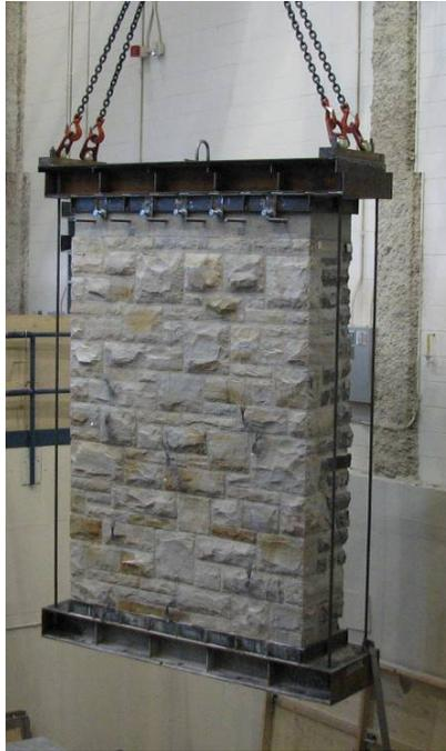
**Figure 3** The lifting system designed for the walls. The base beam and the top beam are connected with four Dywidag bars visible connecting the outer corners of the beams, the system slightly stressed and the wall lifted.
