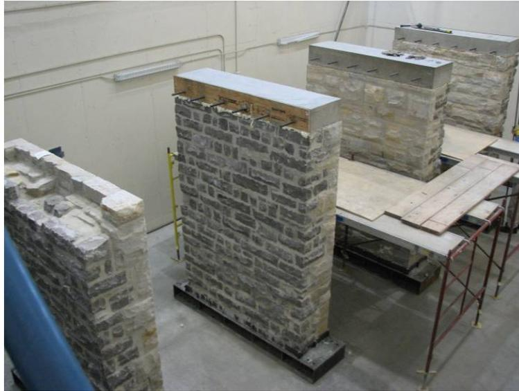
**Figure 1** The walls after casting the concrete cap. Sandstone faces are visible in the two walls to the right of the figure, and limestone faces on the two walls to the left.
