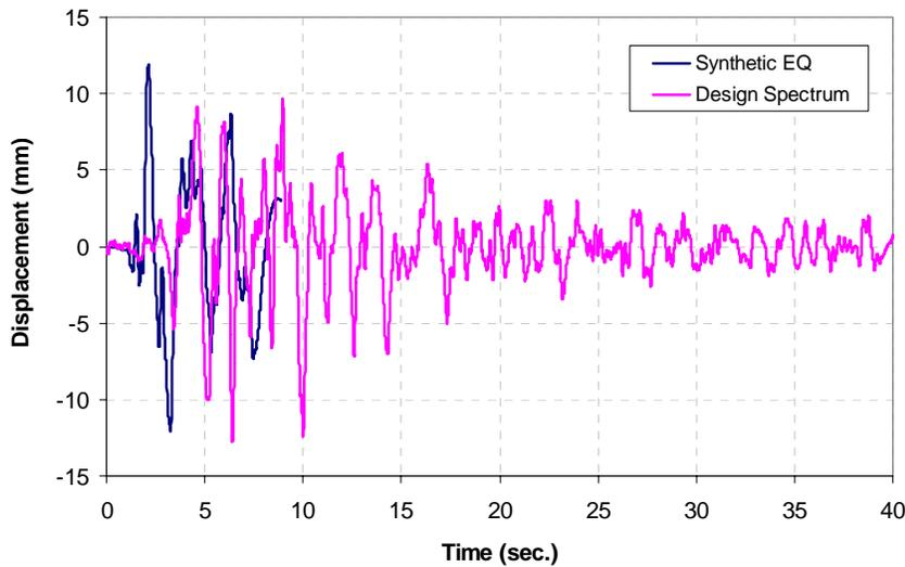
**Figure 7** The earthquakes simulated by the shake table.
