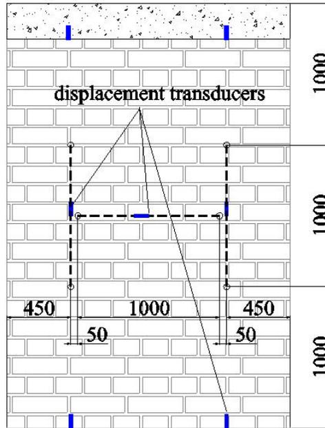
**Figure 5** The instrumentation on each side of the wall for compression testing
