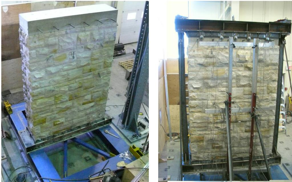
**Figure 6** A wall placed on the shake table (left) and the frame designed to restrain its movement and its instrumentation on the shake table (right).
