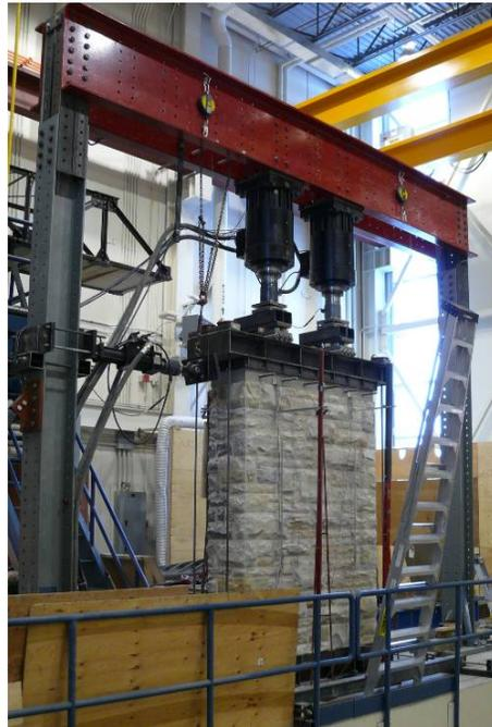
**Figure 4** Schematic of the testing rig above, showing the two actuators at the top and one actuator to the side for lateral loading. A wall is shown in the rig in the picture below.
