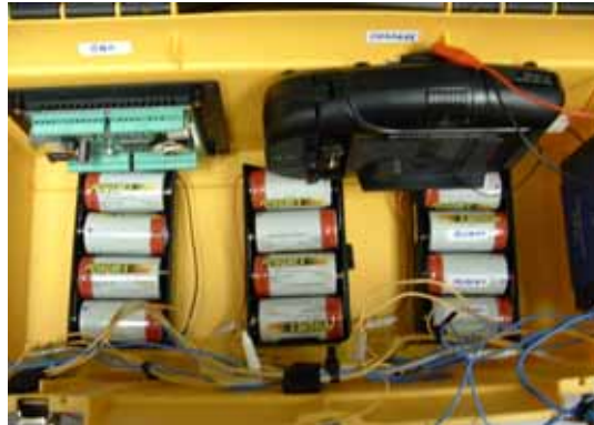
Figure 4. Separate Power Supplies for Z-World Single IC board, Crossbow Accelerometer, and Linksys Wireless Ethernet Bridge [10].
