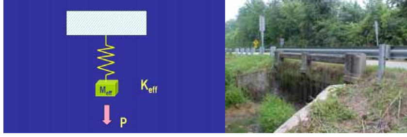
Figure 2. Bridge Modeled as Mass-Loaded Spring.
