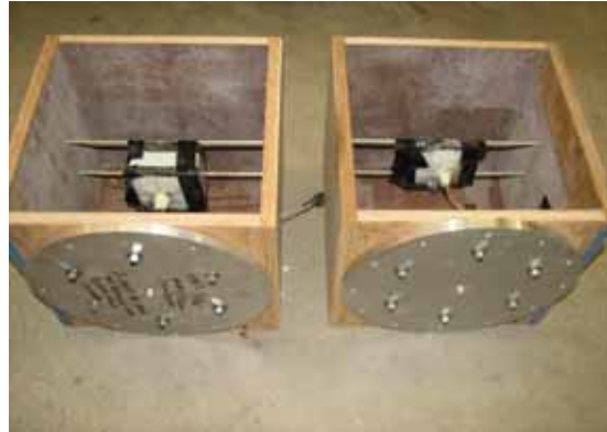
Figure 8. Fabricated antennas placed inside a wooden cast. The wires coming out of the box are used for gain measurements after the concrete has been poured.
