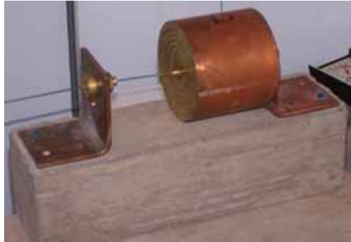
Figure 7 Wireless displacement sensor mounted onto concrete test prism for temperature sensitivity testing.
