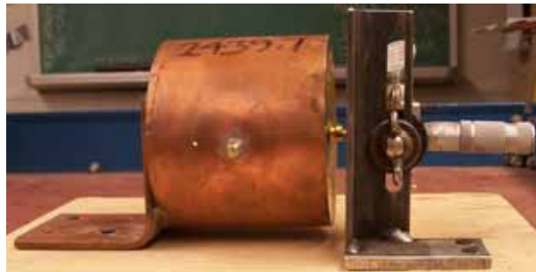
Figure 5. The displacement sensor was mounted on a test jig and a wire was attached to the diaphragm. Using the micrometer the diaphragm was translated in 0.1 mm increments. At each increment the resonant frequency of the cavity was determined using the servo method outlined above.
