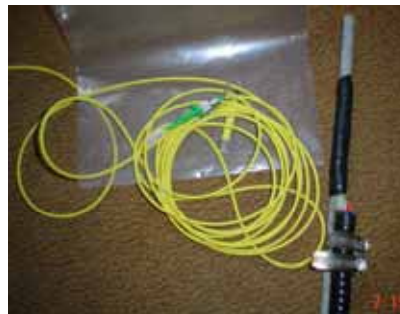
Figure 5. An FBG Optical Sensor
