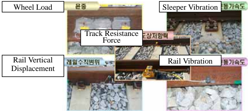
Figure 4. Track Measurement for Status Evaluation (Korea)
