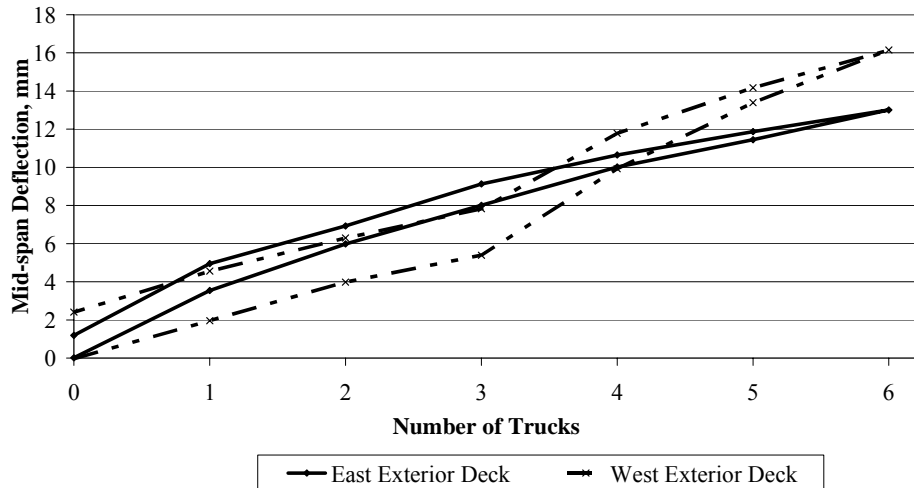
Figure 10: Midspan deflection of exterior concrete deck slab panels for loading and unloading cycles
