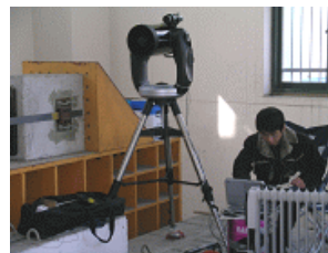
(c) “Non-contact” displacement measurement
