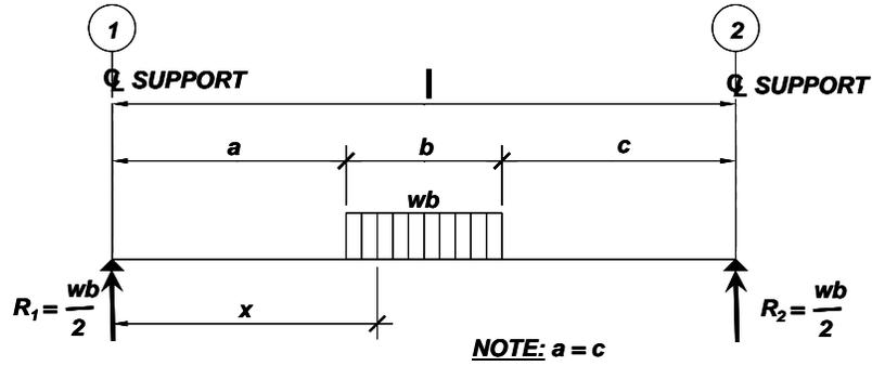
Figure 5: Idealized view of simply supported pre-stressed girder test set-up
