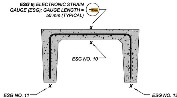
Figure 4b: Locations of electronic strain gauges on cross-section 'C' from Figure 4a
