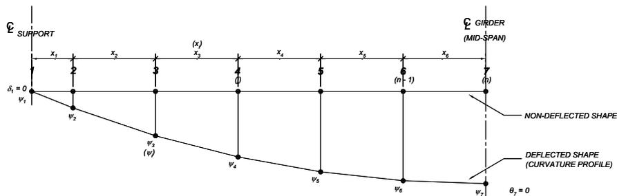
Figure 6: Simplified profile of simply supported girder illustrating principle of numerical integration
