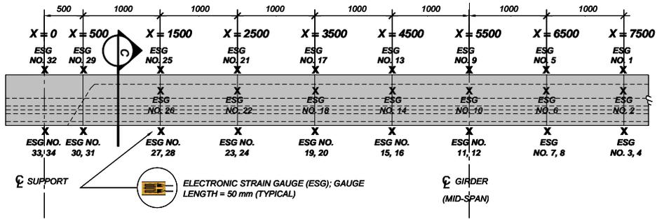
Figure 4a: Locations of electronic strain gauges along the girder
