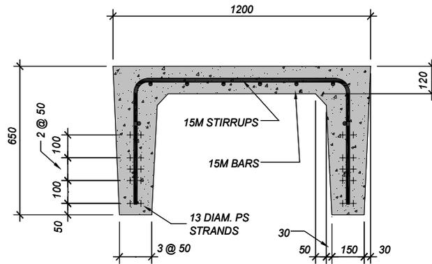
Figure 1: Typical cross-section of full-scale pre-stressed concrete bridge girder (all dimensions shown in mm)
