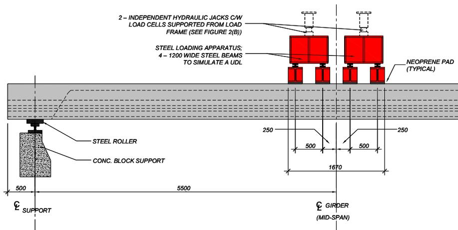
Figure 2a: Elevation of simply-supported beam and loading apparatus
