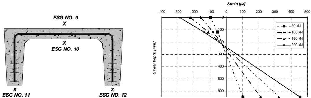
Figure 7: Plot of strain versus depth of girder for strain gauges located at mid-span of the pre-stressed concrete girder.
