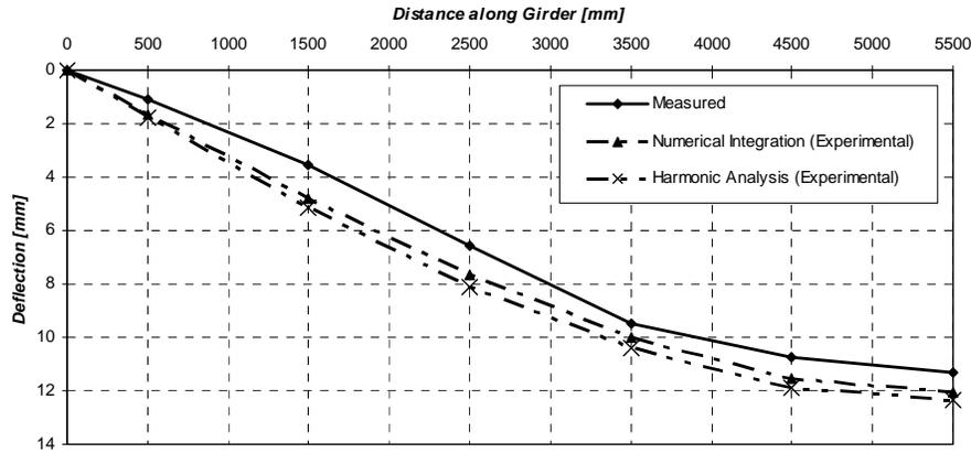
Note: Deflection profiles shown are for one half of the pre-stressed concrete girder. Symmetry was assumed.
