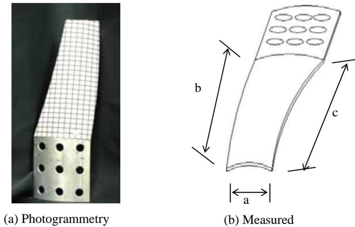
Fig. 3. Warped plate
