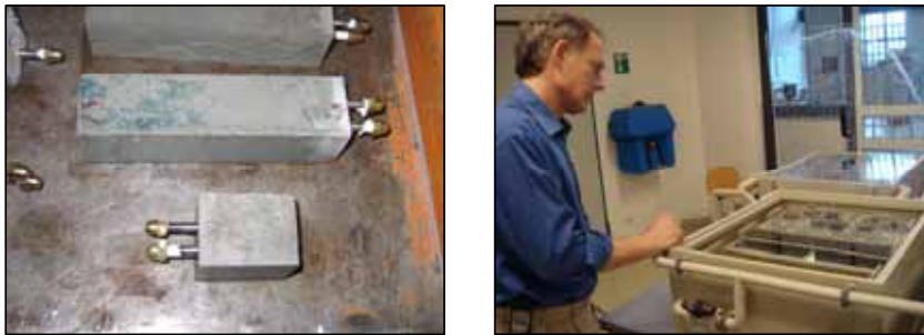
Figure 11. Mortar test samples with integrated sensors (left); acid bath for simulating environmental attack (right).
