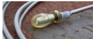
Figure 10. Fixing of the pH sensors in the prefabricated anchors. To prevent dehydration of the pH sensitive membrane, the sensor head is protected by a topcoat (right).
