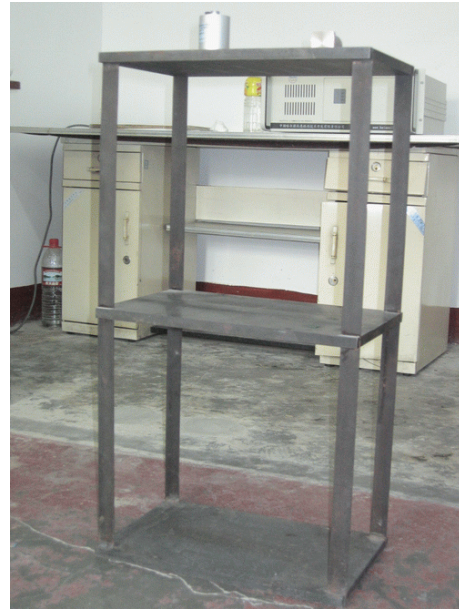
Fig. 10 Photo of Two-story Steel Frame Structure Model
