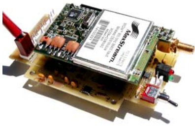
Figure 1. Fully assembled wireless sensing unit prototype (battery and external container not shown for clarity).
