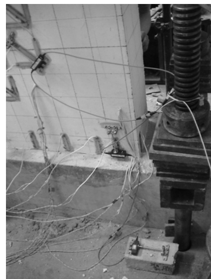
Figure 5. Surfaced FBG strain sensors
