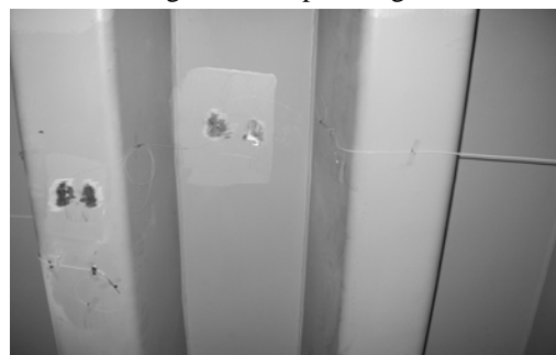
Figure 12. FBG sensors being placed
