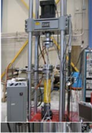
Figure 5. Experimental test setup with coupon in MTS machine.
