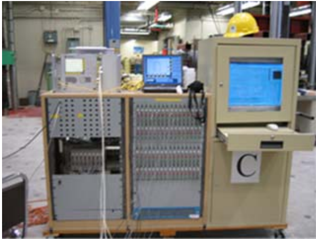
Figure 6. Electrical and optical sensor data acquisition systems.
