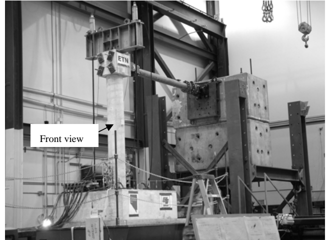
Figure 1. Shaketable, specimen, and mass rig test setup
