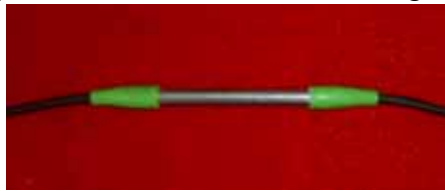
a) Metal tube packaged temperature sensor
