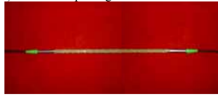
c) FRP packaged FBG strain sensor
