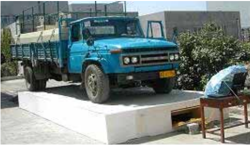
Figure 18. High durable traffic Weighbridge based on FBG sensors
