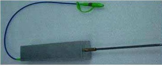
Figure 12. FBG displacement meter developed at HIT
