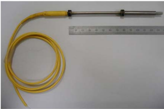
Figure 4 Photograph of the steel tube-based ESPS
