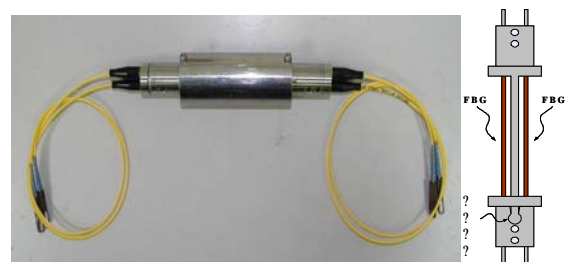
Figure 3. Aspect of POFC's FBG bending sensor
