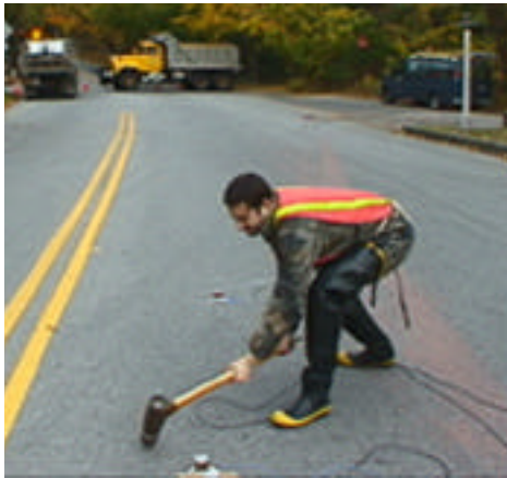
Figure 6: Impact testing of a T-beam bridge
